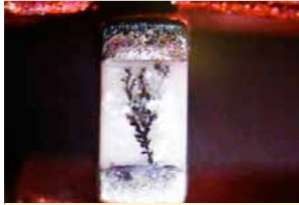
Figure 2. Dendritic growth on component with 5 VDC applied (courtesy Foresite).
